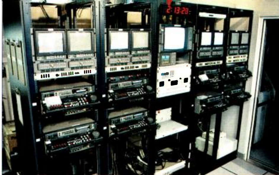
Included in WLWT's rack room are Panasonic DVCPRO decks for recording and playback tasks.
